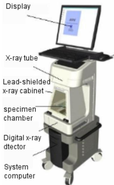
Fig. 1 – A typical intra-operative specimen radiography system (Bioptics, Inc. Tucson, AZ)
